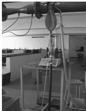
Figure 3: Photograph of Experimental Model from Front Showing the Pipe Connections and Collapsible Bladder
